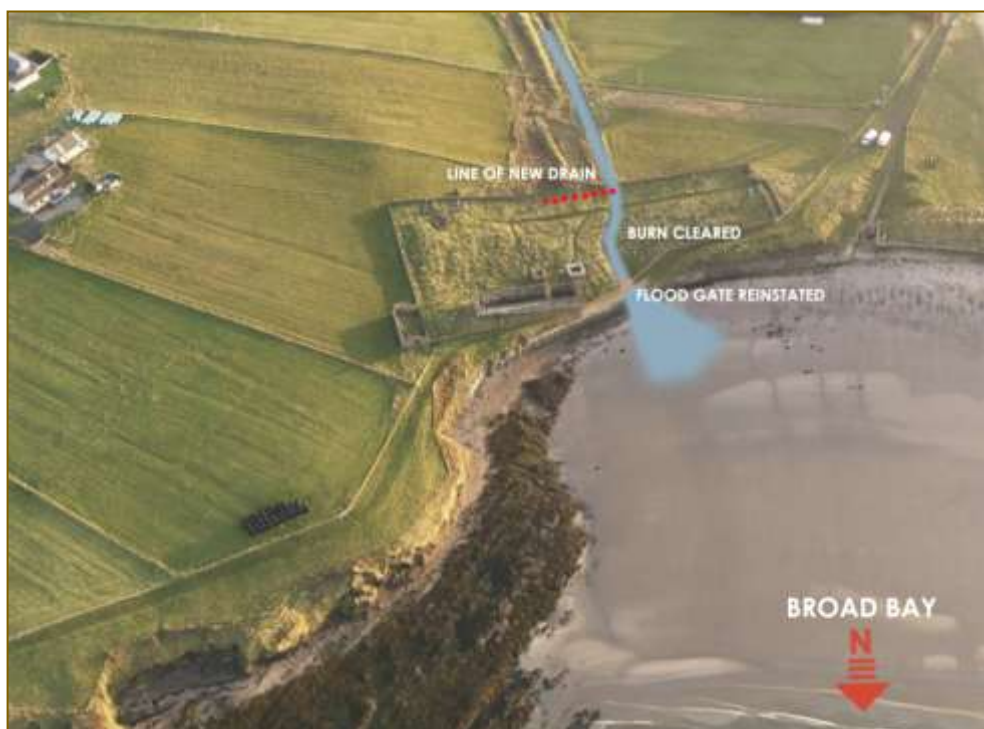
PROPOSED DRAINAGE IMPROVEMENTS
